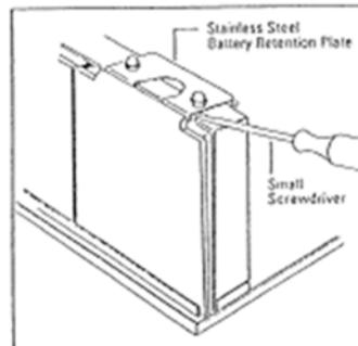
**Step 2.** With the battery removed, adjust both sides of the battery retention plate. Using pliers, slightly raise the bent edges. Adjust the bent edges of the plate so the battery remains secure but can easily be removed.
